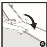
**4** Insert the end of the second board into the end of the first, pressing them together and pushing gently down towards the floor. Complete the first row in the same manner.
