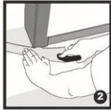
**2** Door Frames: saw the doorframe, resting the flat edge of the saw against a board so that the board can fit underneath.
