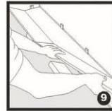
**9** Place the end of the second board against the end of the first board and fit them together by pressing down towards the floor. Be sure to correctly align the boards, and position another triangular wedge.
