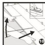
**10** Continue in this way with the whole row. Be sure that the strip is driven well into the groove, and press the boards strongly towards the floor so as to fit them together. Remove the wedges at the same time.
