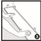
**3** Lay the first board against the left wall, with the tongue-side towards the wall. Make sure you leave a space of 8 to 10 mm/ 1/3 to 3/8", to allow for expansion. If the wall is uneven, the boards should be sawn and adapted to the contour of the wall.
