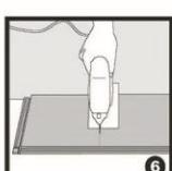
**6** To cut the boards, place them face down against the work surface and cut to the desired shape using a jigsaw. If using a traditional hand saw, place the board face up and use a fine-toothed blade.
