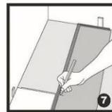
**7** Start the second row by using the leftover part of the board you have sawn. It should be at least 30 cm / 10" long. If not, use a new board, cutting it into two. Make sure that the end joints are always least 30-cm/ 10" apart.
