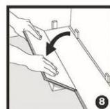
**8** Place the sawn board by tilting it against the first row board Exert pressure and, at the same time, press down towards the floor. Place a triangular wedge under the board.
