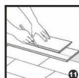
**11** Before laying the final row, measure and saw the board accordingly. Leave 8 to 10 mm / 1/3 to 3/8" gap between the board and the wall to allow for any expansion.
