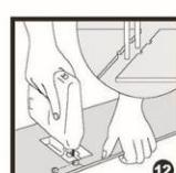
**12** Pipes. Measure the diameter of the pipe and allow for an extra 10 mm / 3/8" leeway. After cutting the board as illustrated in the diagram below, lay the board and the part sawn off.
