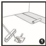
**1** To start, ensure that no damage has been done to the flooring during transportation. After cleaning the floor surface you can roll out the plastic sheet and underlay material. The plastic sheet should overlap by at least 20 cm/ 8".
