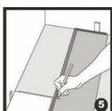
**5** At the end of the row, place the last board face down, with the short side (side without the groove) facing the wall. Mark the floorboard where it has to be cut, making sure to leave a space of 8 to 10-mm/ 1/3 to 3/8" to allow for expansion.
